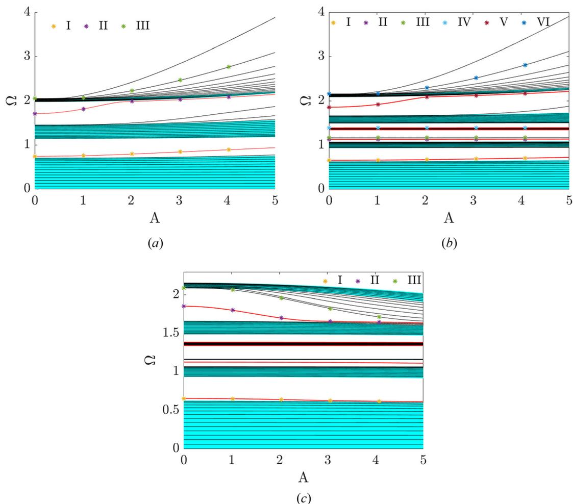
**Fig. 3** Effect of excitation amplitude  $A$  on the dispersion relations of a nonlinear chain at phase  $\phi = 0.35\pi$  (a) without resonators, (b) with resonators and hardening nonlinearity,  $\epsilon = 0.1$ , and (c) with resonators and softening nonlinearity,  $\epsilon = -0.1$
