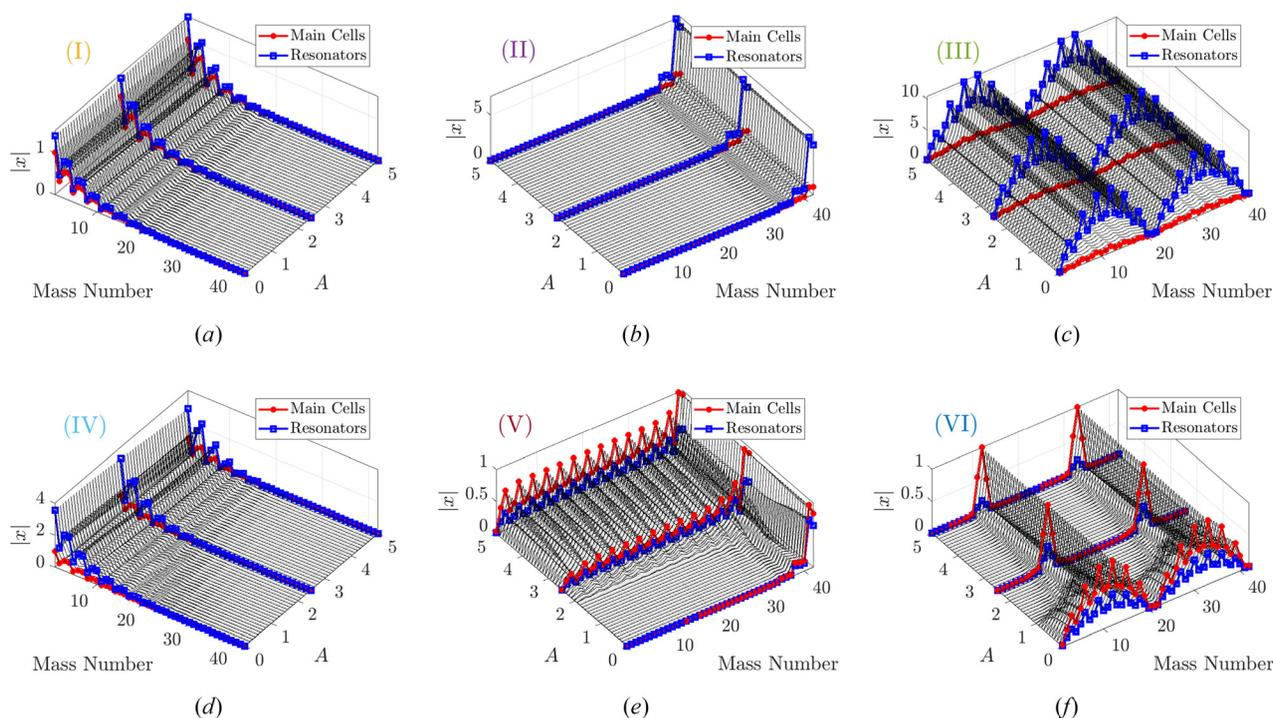
**Fig. 6** Effect of excitation amplitude  $A$  on selected mode shapes of a hardening nonlinear chain ( $\epsilon = 0.1$ ) with  $N = 42$  masses, with resonators, and  $\phi = 0.35\pi$ . (a) mode 15 (1st edge mode); (b) mode 29 (2nd edge mode); (c) mode 41; (d) mode 57 (3rd edge mode); (e) mode 71 (4th edge mode); and (f) mode 83.
