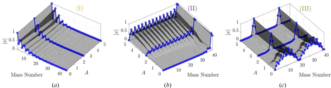
**Fig. 5** Effect of excitation amplitude  $A$  on selected mode shapes of a hardening nonlinear chain ( $\epsilon = 0.1$ ) with  $N = 42$  masses, without resonators, and  $\phi = 0.35\pi$ . (a) mode 15 (1st edge mode); (b) mode 29 (2nd edge mode); and (c) mode 41.
