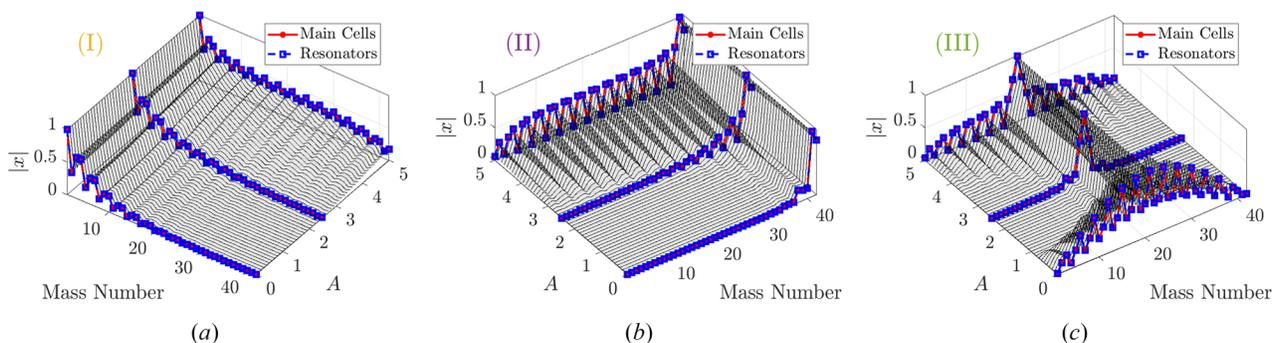
**Fig. 8** Effect of excitation amplitude  $A$  on selected mode shapes of a softening nonlinear chain ( $\epsilon = -0.1$ ) with  $N = 42$  masses, with resonators, and  $\phi = 0.35\pi$ . (a) mode 15 (1st edge mode); (b) mode 71 (4th edge mode); and (c) mode 72.
