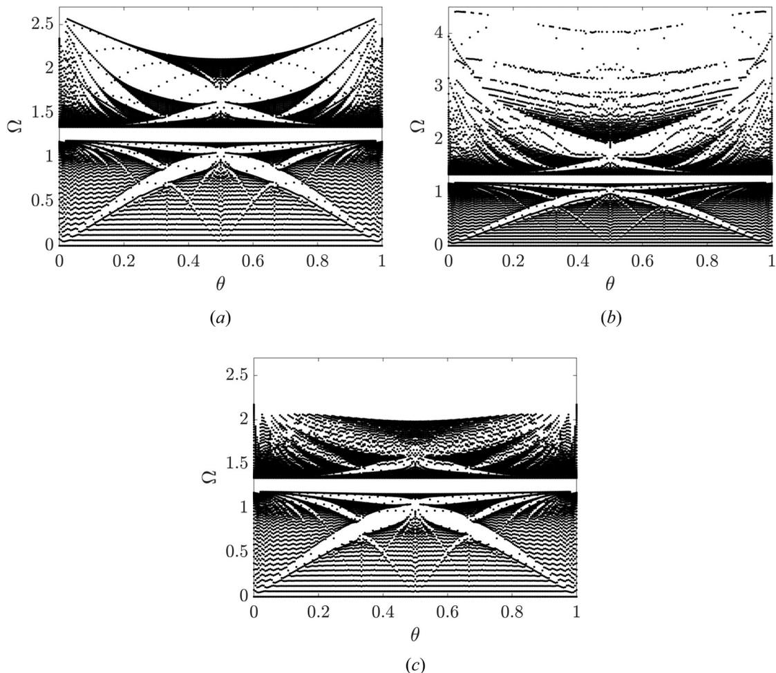
**Fig. 4** Natural frequency spectrum plotted over a range of quasi-periodic parameters,  $\theta$ , with hardening nonlinearity,  $\epsilon = 0.1$ , at (a) low amplitude,  $A = 0$  and (b) high amplitude,  $A = 5$
