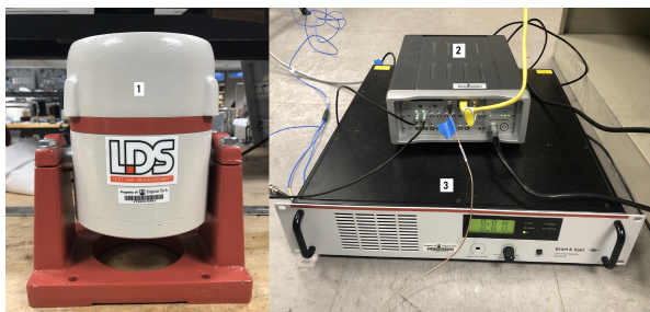
FIGURE 3: Experiment hardware. (1) exciter, (2) analyzer, (3) signal conditioner.
