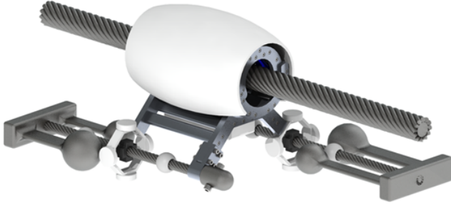
FIGURE 1: Conceptual design model of the mobile damping robot.
