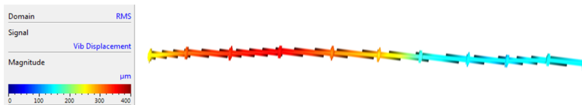
Figure 2.18: Displacement for the same cable segment with a mass corresponding to 15% of the cable mass attached at an antinode (A3).
