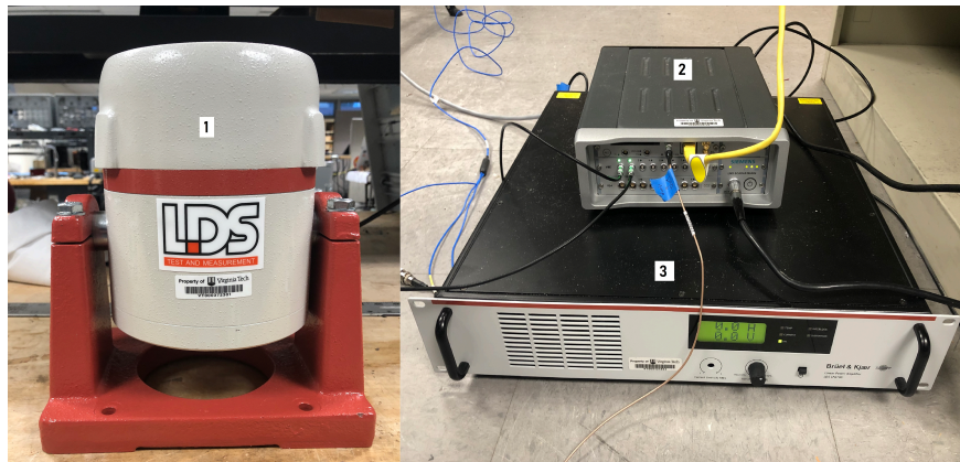
Figure 2.3: Experiment hardware. (1) exciter, (2) analyzer, (3) signal conditioner.
