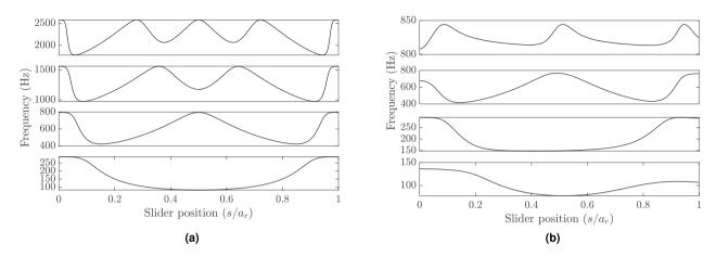
Figure 2. The lowest four resonance frequencies at different slider positions: (a) Slider beam only; (b) combined system.
