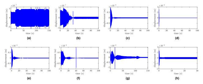
**Figure 6.** Tip displacement of the primary structure at different excitation frequencies: (a) f = 78 Hz,  $w_0 = 0.1g$ ; (b) f = 85 Hz,  $w_0 = 0.1g$ ; (c) f = 130 Hz,  $w_0 = 0.1g$ ; (d) f = 140 Hz,  $w_0 = 0.1g$ ; (e) f = 150 Hz,  $w_0 = 0.1g$ ; (f) f = 155 Hz,  $w_0 = 0.1g$ ; (j) f = 200 Hz,  $w_0 = 0.5g$ ; (h) f = 250 Hz,  $w_0 = 0.8g$ .
