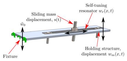
Figure 1. Key components of the self-tuning vibration absorber installed on a structure.
