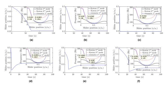
**Figure 7.** Slider position at different excitation frequencies: (a) f = 110 Hz,  $w_0 = 0.1g$ ; (b) f = 130 Hz,  $w_0 = 0.1g$ ; (c) f = 140 Hz,  $w_0 = 0.1g$ ; (d) f = 145 Hz,  $w_0 = 0.1g$ ; (e) f = 150 Hz,  $w_0 = 0.1g$ ; (f) f = 155 Hz,  $w_0 = 0.1g$ .
