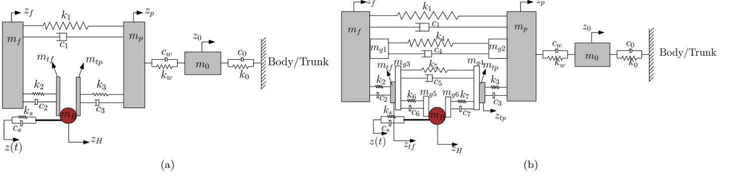
Figure 1: Schematic of hand-arm system (a) without glove, and (b) with glove.
