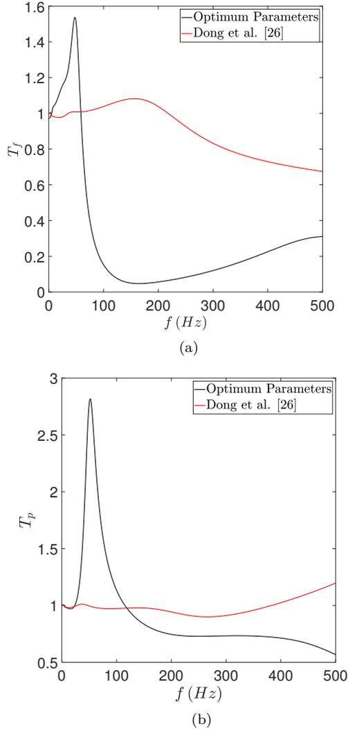
Figure 5: Comparison of relative (a) finger transmissibility (b) palm transmissibility curves for the optimum glove parameters and glove parameters used in [26].
