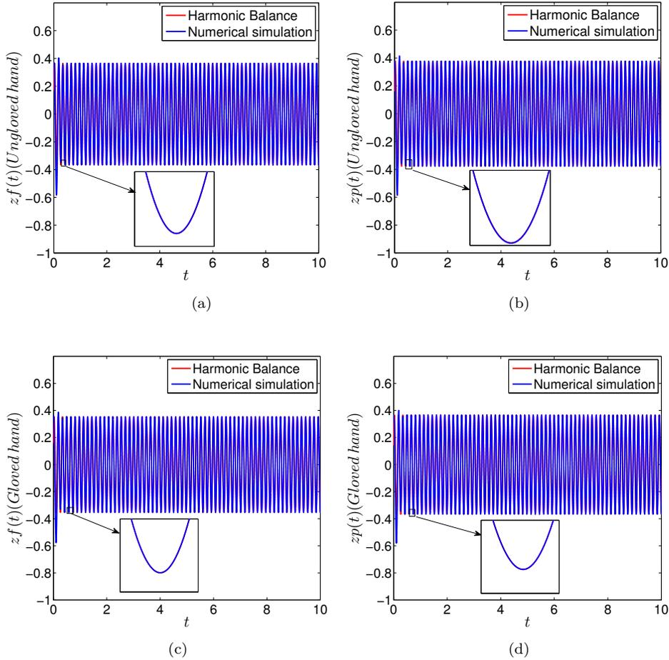
Figure 2: Responses of (a) fingers without gloves, (b) palm without gloves, (c) fingers with gloves, and (d) palm with gloves. The other parameters are chosen as  $Z_0 = 1$ ,  $m_{g2} = m_{g1}$ ,  $m_{g4} = m_{g3}$ ,  $m_{g6} = m_{g5}$ ,  $k_7 = k_6$  and  $c_7 = c_6$
