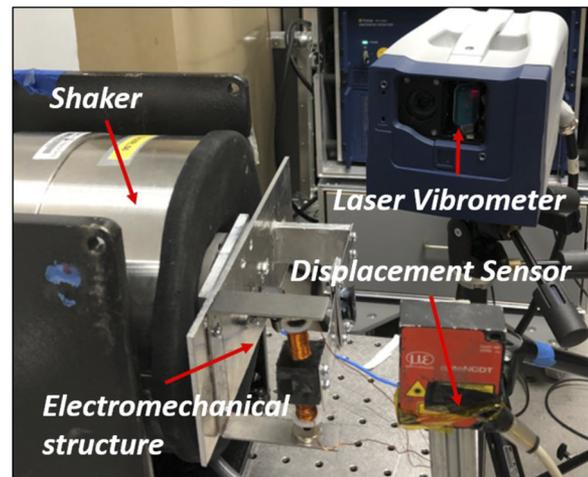
FIG. 5. Key components of the experimental setup.
