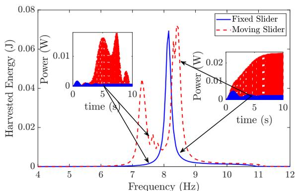
FIG. 4. Total energy harvested over 10 s with and without a sliding mass for a range of frequencies  $s_0 = 0.5L$ .
