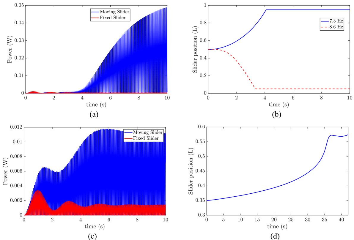
**FIG. 3.** Simulation results at different excitation frequencies: (a) Harvested power at 7.3 Hz; (b) slider position at 7.3 Hz and 8.6 Hz; (c) harvested power at 8.6 Hz; and (d) slider position at frequencies close to the second vibration mode at 72.2 Hz.
