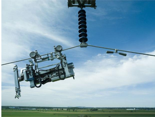
Figure 1.9: Hydro Quebec Linescout inspection robot
