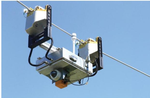
Figure 1.10: The transmission line inspection robot developed by EPRI.
